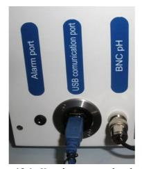
Figure 19.1 pH probe connected to the BNC
